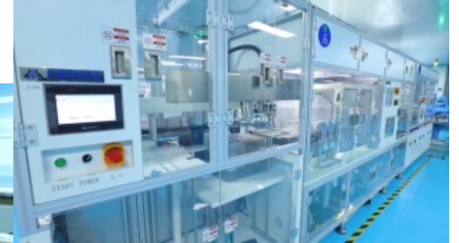
Polarizer & glass bonding line
